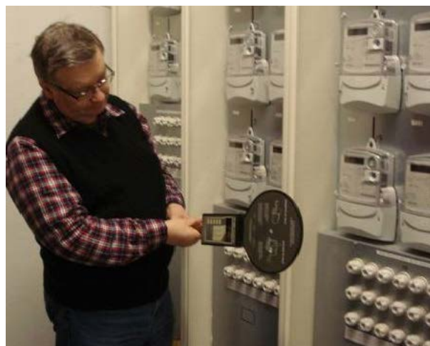
Figure 2. Example of electric field measurement at 30 cm distance
