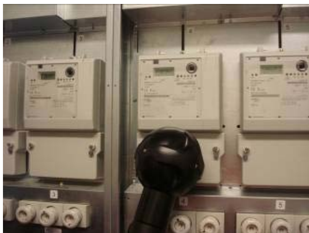
Figure 3. Example of magnetic field measurement at surface of meter
