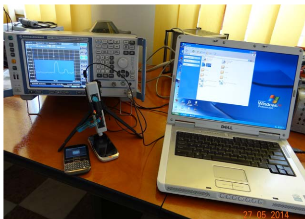
Figure 1. Experimental set-up with the E-field probe inspecting the phones and the real-time signal analyzer during 3G-phones' scan
