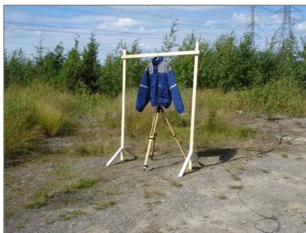
Figure 3. Winter jacket in electric field measurement.
