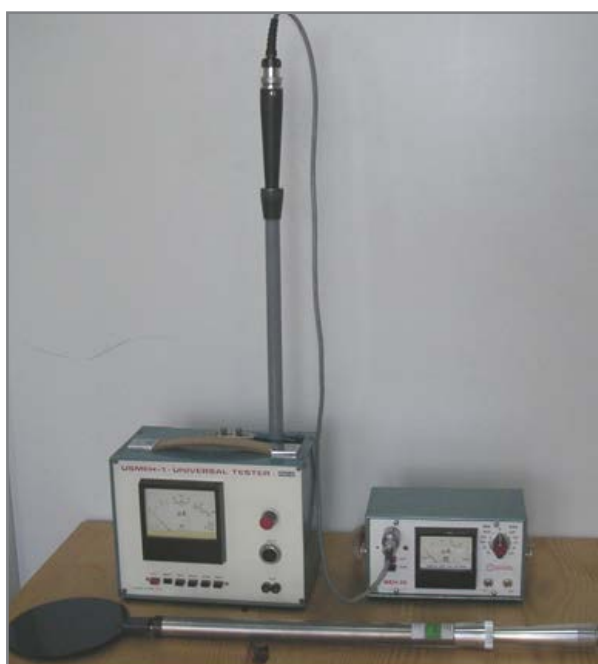
Figure 1. MEH-type EMF meter validation in ISMEH-1 tester.
