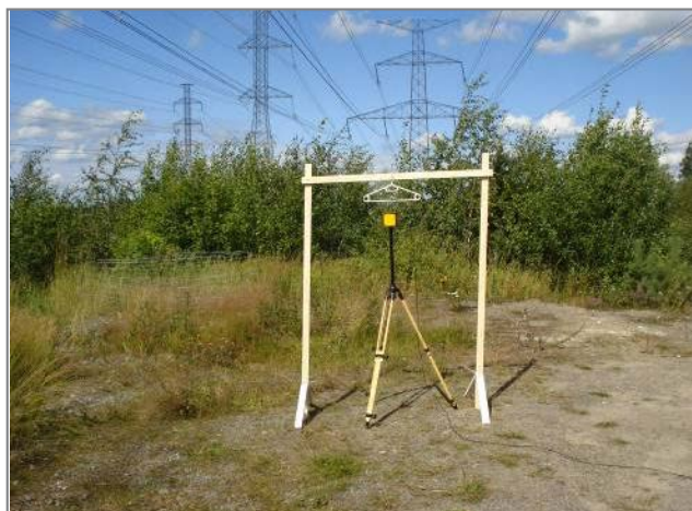
Figure 1. Frame with hanger and electric field meter in measurement location
