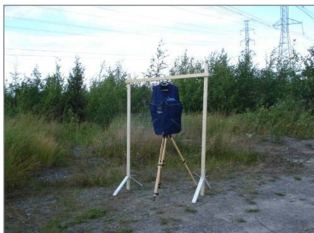
Figure 4. Vest in electric field measurement.
