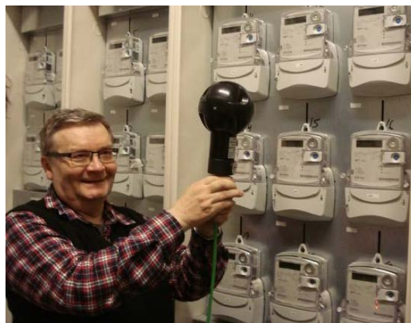
Figure 4. Example of magnetic field measurement at 30 cm distance.
