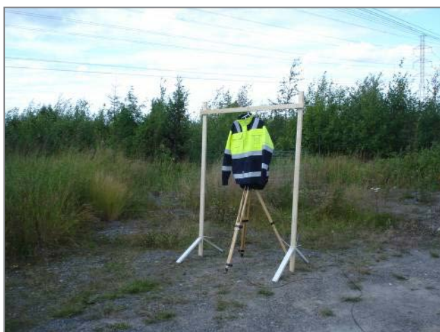
Figure 2. Summer jacket electric field measurement
