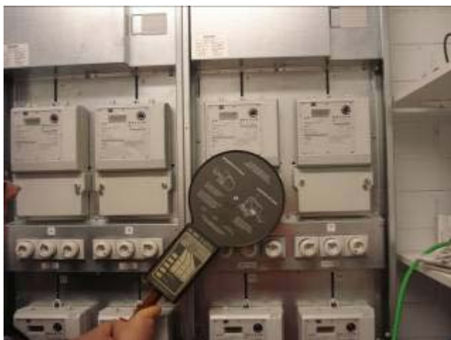
Figure 1. Example of electric field measurement at surface of meter
