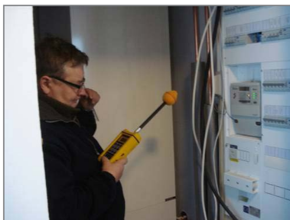
Figure 1. Example of measurement at distance of 30 cm.
