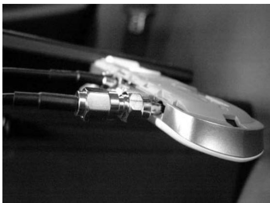
Figure 4. External antennas were connected to the wireless adapter via one or two CRC9 type sockets.
