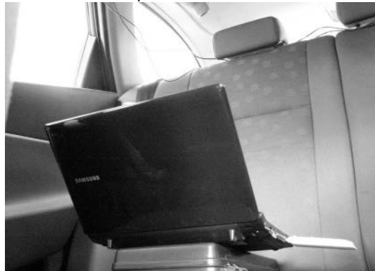
Figure 3. Measurement setup – a PC connected to a wireless network adapter; no external antenna is used in original exposure scenario.
